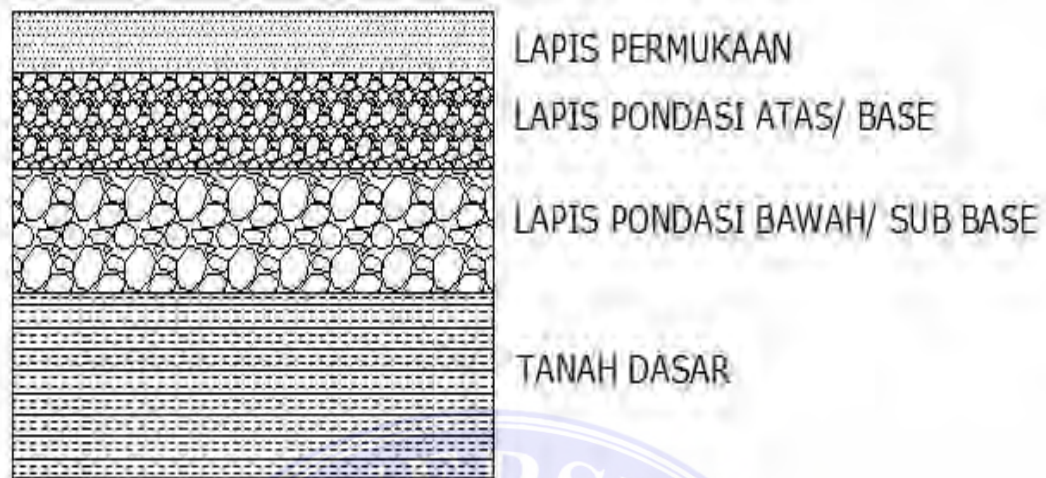
Gambar 2. Lapisan perkerasan lentur (Mubarak,2016)
