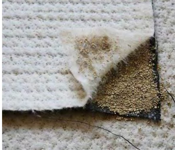
Gambar 8. Geosynthetic Clay liner (Departemen PU, 2009)
