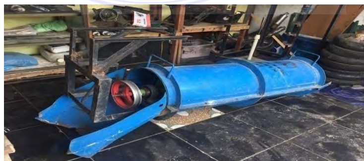
Gambar 3. 1 Turbin Ulir Archimedes screw
