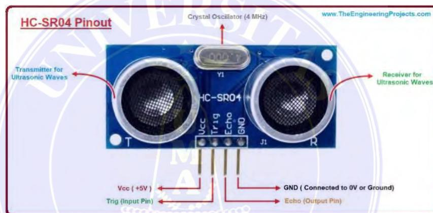
Gambar 2.9 Bagian-bagian Sensor Ultrasonik
