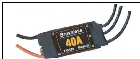
Gambar 2.5 Electronic speed controller Sumber : ( https://images.tokopedia.net/img/cache/700/product-1/2019/6/8/2318021/2318021_7698f2da-ac88-4a61-9a20-481332730557_810_810.jpg )
