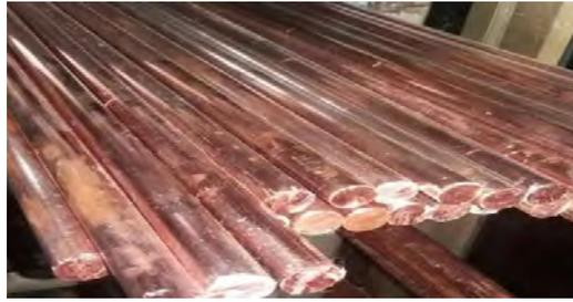
Gambar 2.11 : Elektroda Pentanahan (S-PLN,2014)
