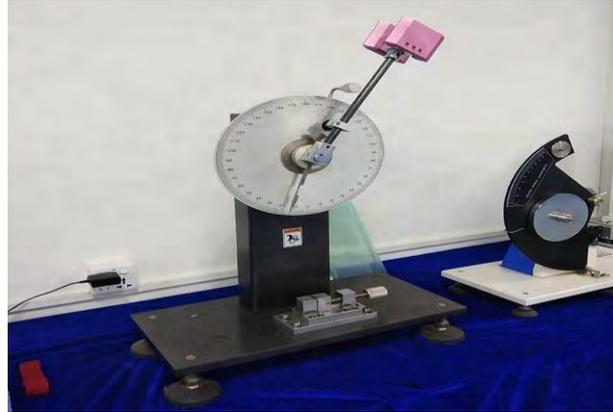
Gambar 2.4. Mesin Impak Charpy.
