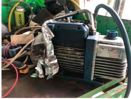
Gambar 3.4 Pompa Vakum
