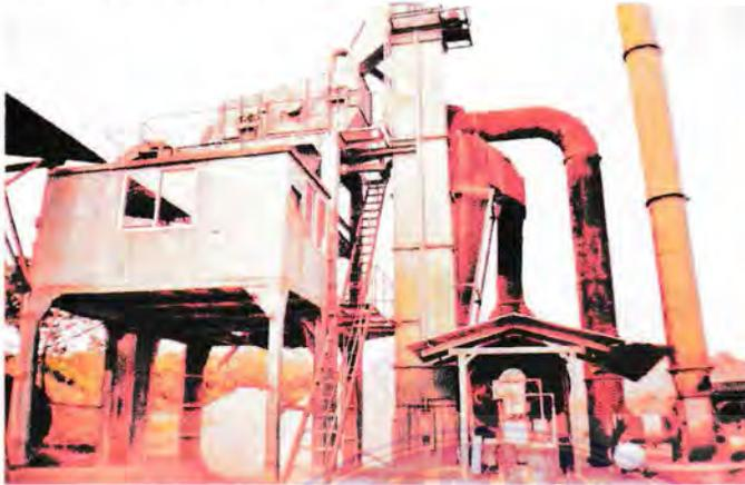
Gambar 2.9 Asphalt Mixing Plant (AMP)
