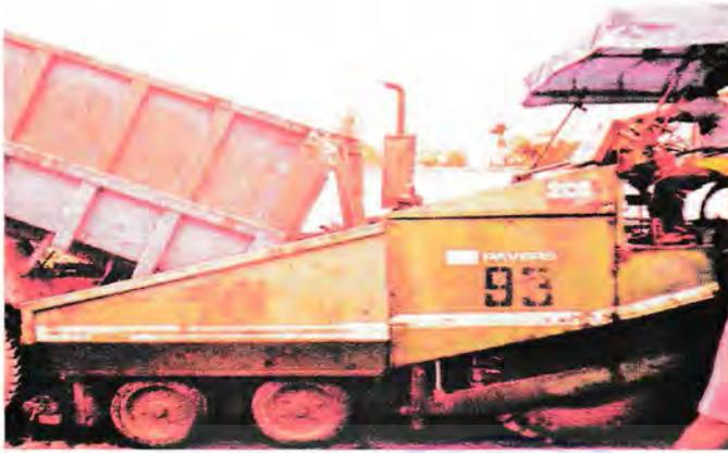
Gambar 2.11 Asphalt Finisher
