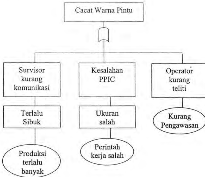
Gambar 5.15. FTA (Fault Tree Analysis ) Cacat Warna Pintu
