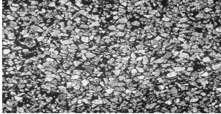
Gambar 14. Agregat licin ( polished aggregate ) (ASTM International, 2018)
