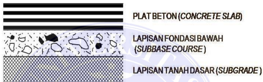
Gambar 2. Lapisan perkerasan kaku (Mubarak, 2016)
