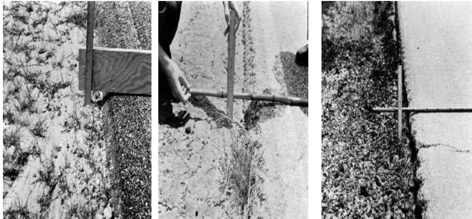
(a) Low (L) (b) Medium (M) (c) High (H) Gambar 9. Pinggiran jalan turun ( Lane/Shoulder drop-off ) (ASTM International, 2018)
