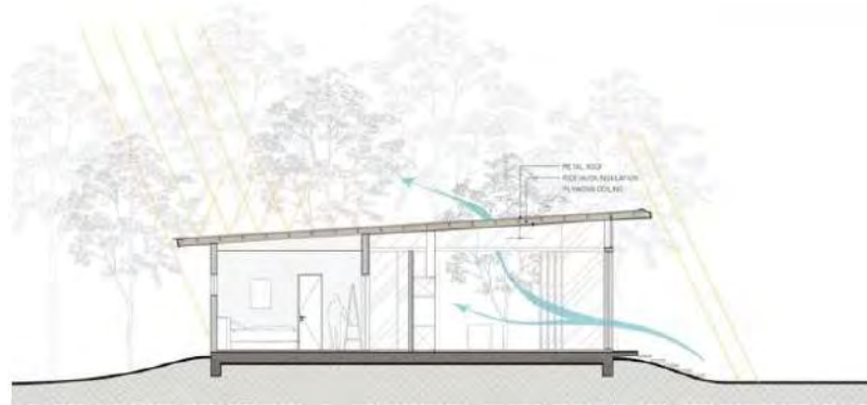
Gambar 2. 13 Sistem Cross Ventilation Tropical Villa
