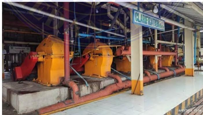
Gambar 3.59 *Sludge Centrifuge*
