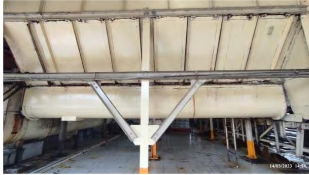
Gambar 3.32 *Under Thresher Conveyor*
