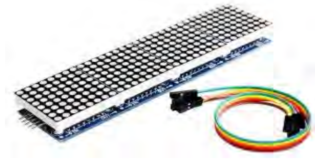
Gambar 2.10: Display LED Dot Matrix (Sumber : https://media.neliti.com/media/publications/191382-ID-perancangan-display-led-dot-matrix-mengg.pdf )
