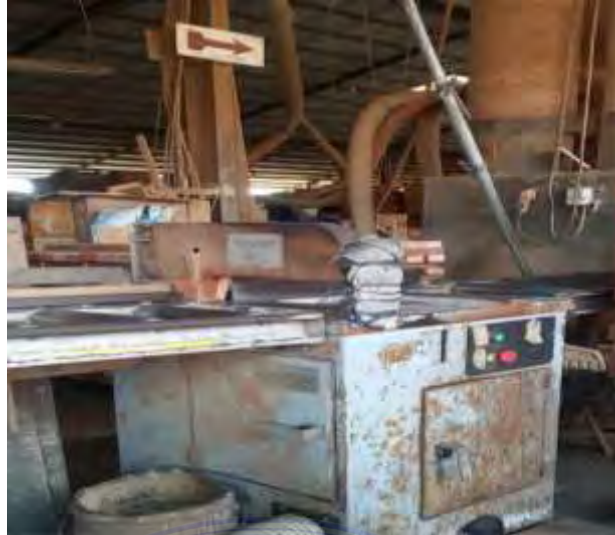
Gambar 3. 14. Under Cut Machine
