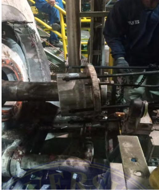
Gambar 3. 15 Pelepasan bearing shaf
