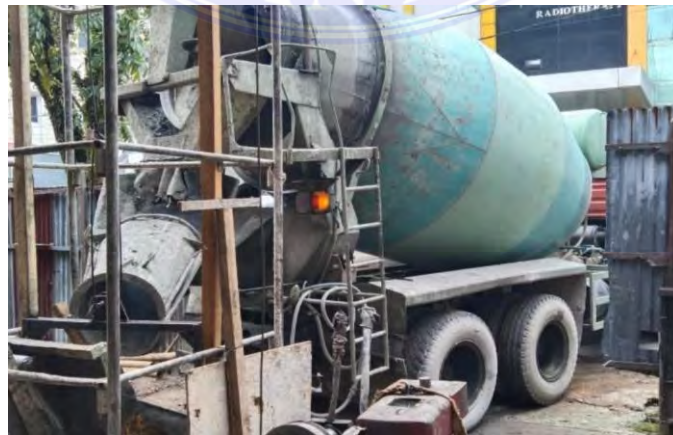
Gambar 3. 8 Truck Mixer Beton Sumber : Data Lapangan
