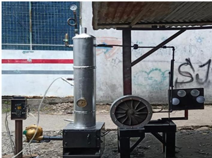
Gambar 3.3. Boiler pipa api skala model
