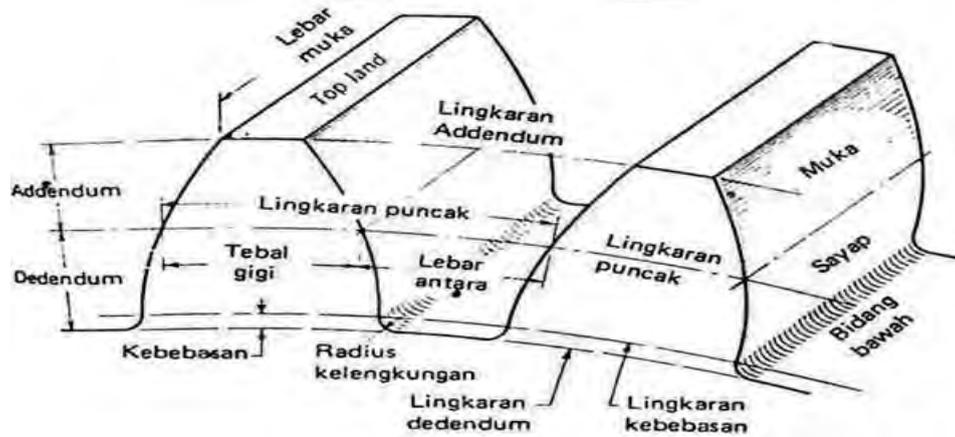
Gambar 2.2. Bagian-Bagian Roda Gigi
