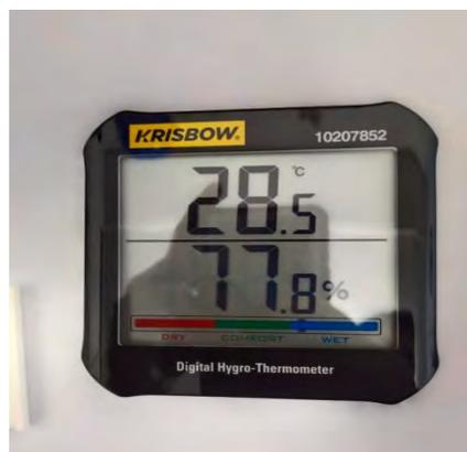
Gambar 2.2. Alat Ukur Kelembaban *Digital Hygro Thermometer*
