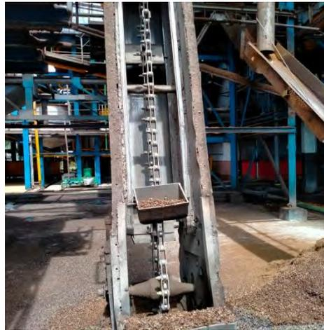
Gambar 3. 38 *Shell Elevator*
