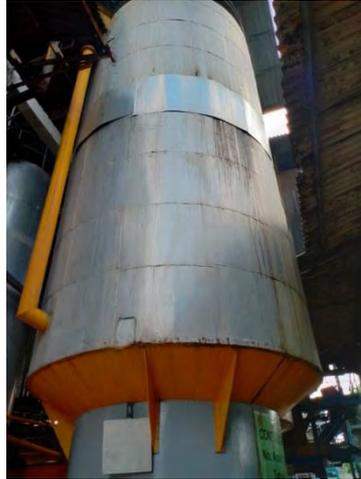
Gambar 3. 20 *Continuous Setting Tank* (CST)
