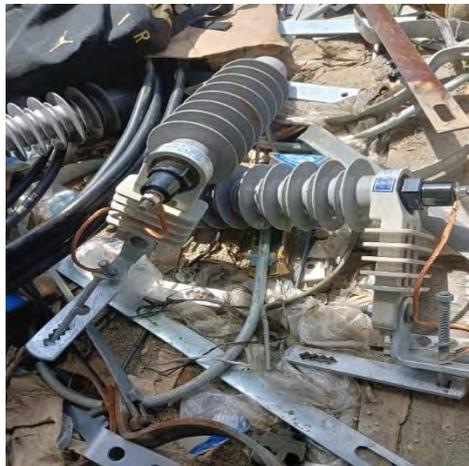
Gambar 2.11 Lightning Arrester
