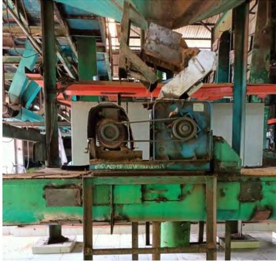
Gambar 3. 38 Ripple Mill
