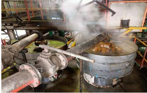
Gambar 3.24 Vibro Sludge Separator
