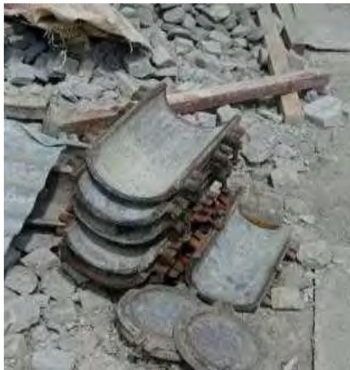
Gambar 3.1.25 Bekisting Silinder Sampel
