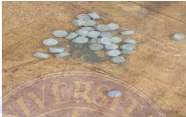
Gambar 3.2.12 Beton Decking
