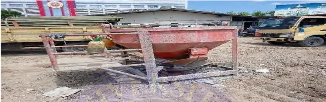
Gambar 3.15 *Concrete Bucket*,
