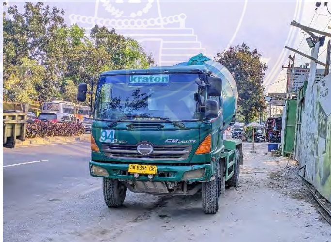
Gambar 3.1.9 Truck Mixer Beton
