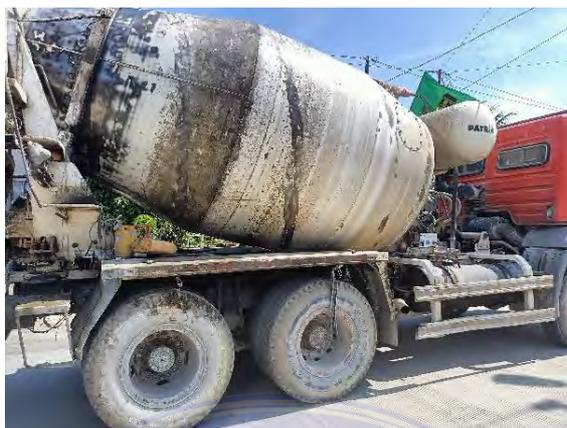
Gambar 3. 8 *Truck Mixer Beton*
