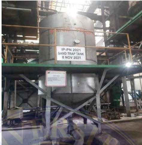
**Gambar 3.25. Sand Trap Tank**
