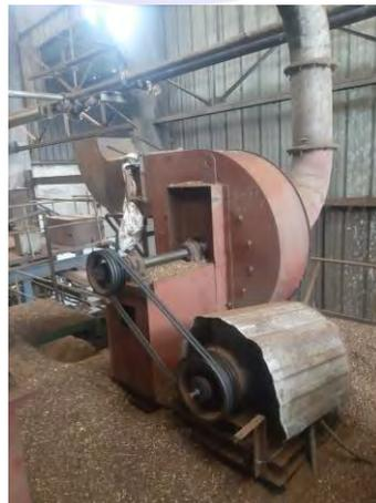
**Gambar 3.20. Ripple Mill**
