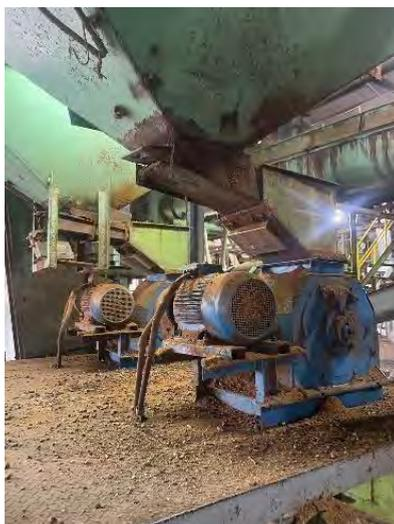
*Gambar 3.27 Ripple Mill*
