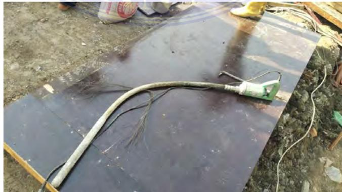
Gambar 3. 3 Beton *Vibrator*
