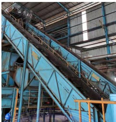
**Gambar 3. 28 Inclined Fruit Bunch Conveyor**
