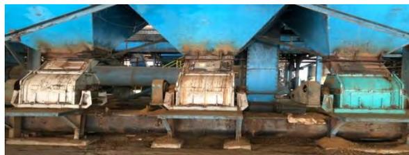
**Gambar 3. 19 Ripple Mill**
