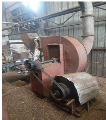
**Gambar 3.20. Ripple Mill**
