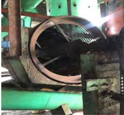
**Gambar 3. 22 Nut Polishing Drum**
