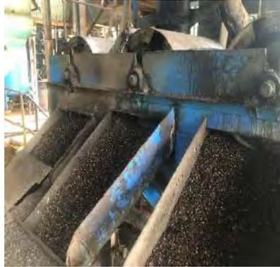
**Gambar 3. 25 Ripple Mill**
