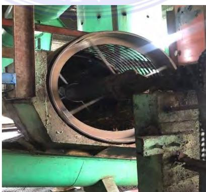
**Gambar 3. 24 Nut Polishing Drum**
