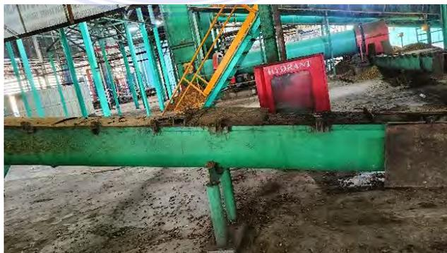
**Gambar 3.24 Wet Nut Conveyor**
