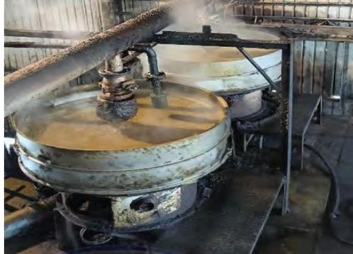
**Gambar 3.40 Vibrating Sludge**
