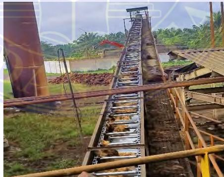
**Gambar 3.13** *Mesin Inclined Empty Bunch Conveyor*
