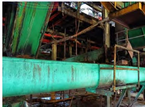
**Gambar 3.11 Mesin *Bottom Cross Conveyor***
