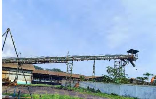
**Gambar 3.12** *Mesin Horizontal Empty Bunch Conveyor*
