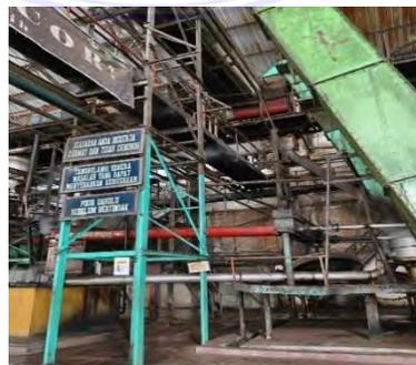
**Gambar 3. 28. Inclined fruit bunch conveyor**
