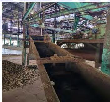
**Gambar 3. 30. Inclide distribusi bunch conveyor**
