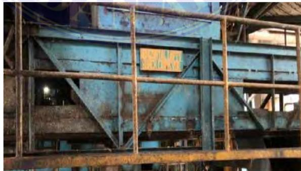
**Gambar 3. 29 *Horizontal Empty Bunch Conveyor***
