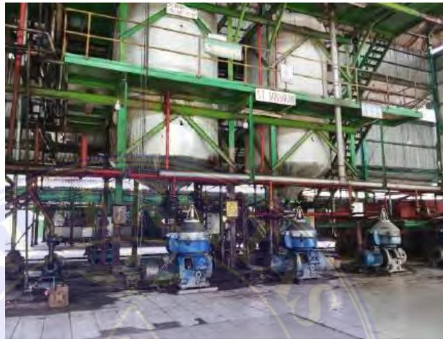
Gambar 3.18. *Sludge Tank*
