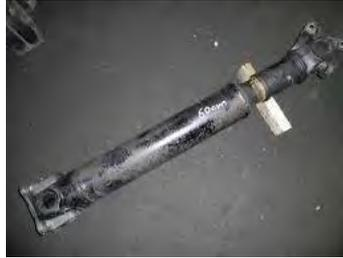
Gambar 3.3. *Propeler Shaft*
