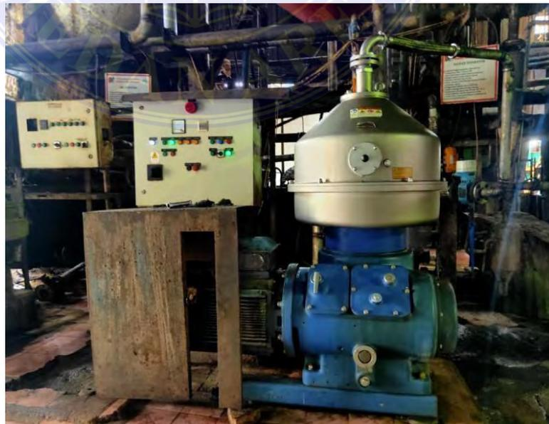
Gambar 3.33. *Sludge Seperator*
