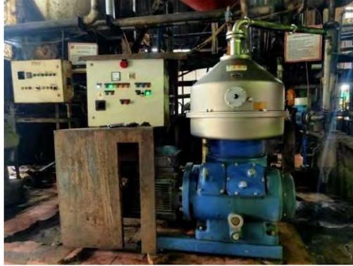
Gambar 3.33. *Sludge Separator*
