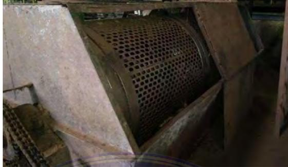
Gambar 3.39. *Nut Grading Drum*
