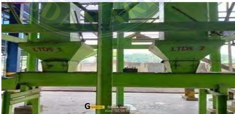
**Gambar 3.14. *Ligh tenera dry separating (LTDS-1)***
