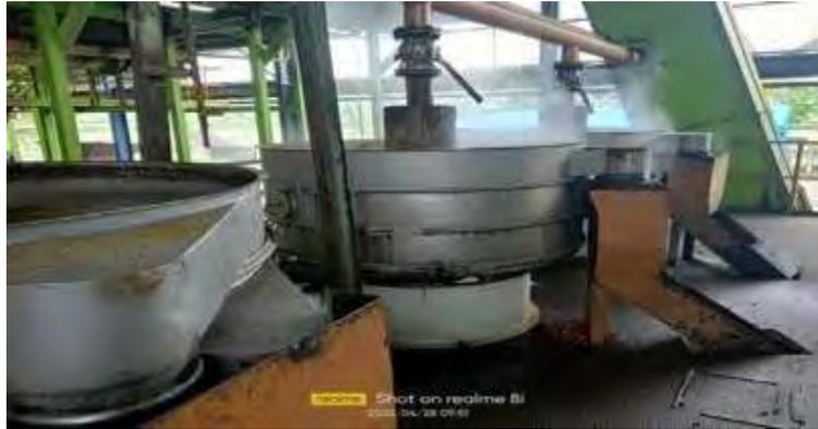
**Gambar 3.30. Oil Vibre Separator**
