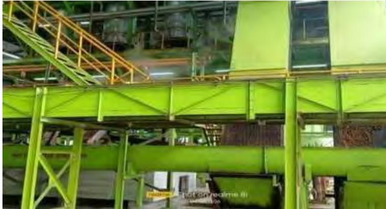
**Gambar 3.28. *Horizontal empty bunch conveyor***
