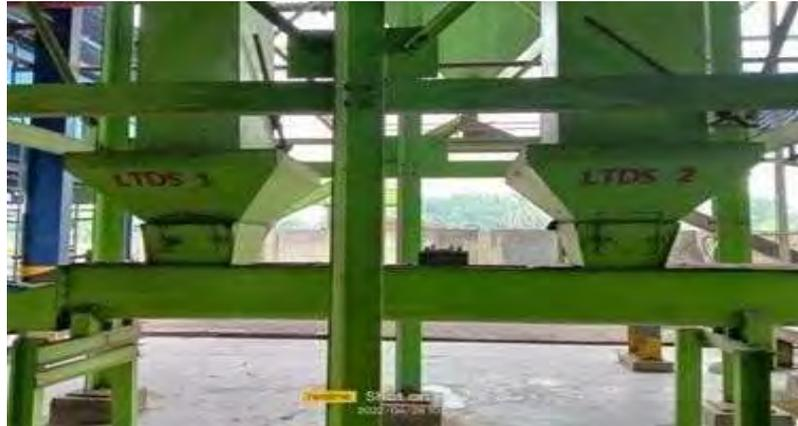
**Gambar 3.15. *Ligh tenera dry separating (LTDS-2)***
