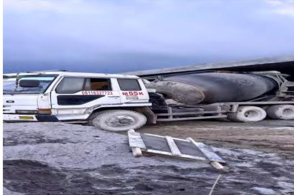
Gambar 3.7 *Truck Mixer Beton*
