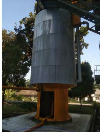
Gambar 3.17. *Continuous Setting Tank*
