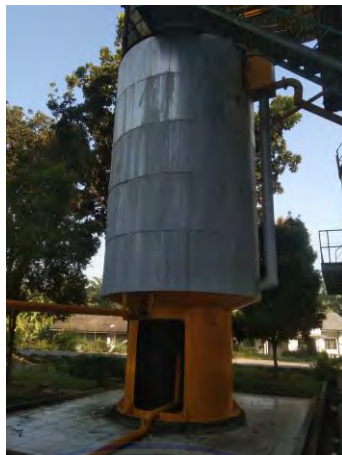
Gambar 3.17. Continuous Setting Tank
