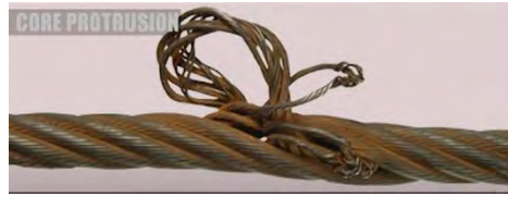
Gambar 3.15. kink, Bridcaging, dan core protrusion
