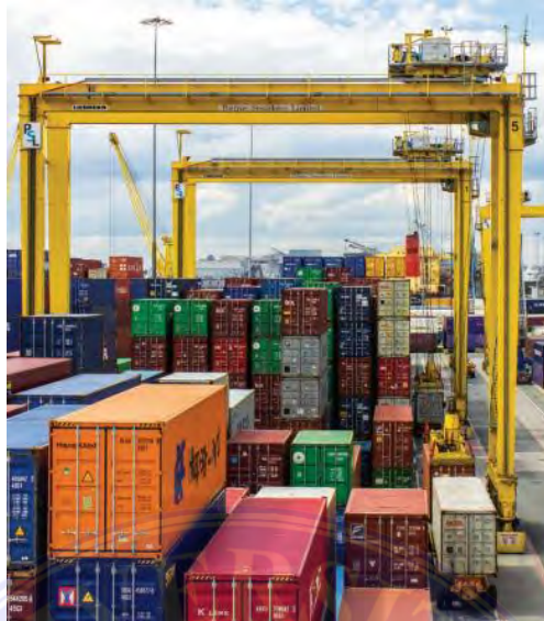
Gambar 3.2. Rubber Tyre Gantry Cranes (Liebherr Ontrainer Cranes)
