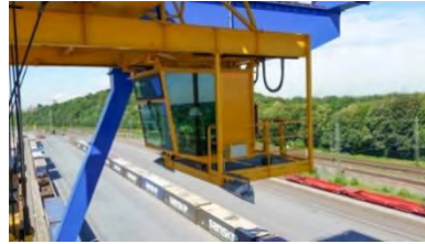
Gambar 3.11. Cabin Operation Control Rubber Tyred Gantry Craner
