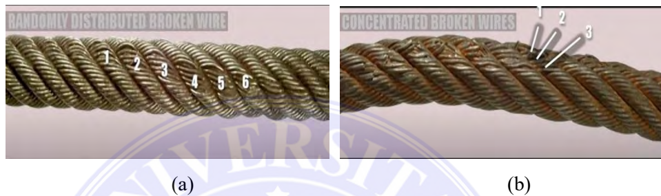
Gambar 3.14. Randomly Distributed Broken wire dan concentrated Broken wire
