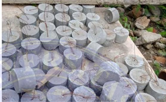
Gambar 3.11 Beton *Decking*
