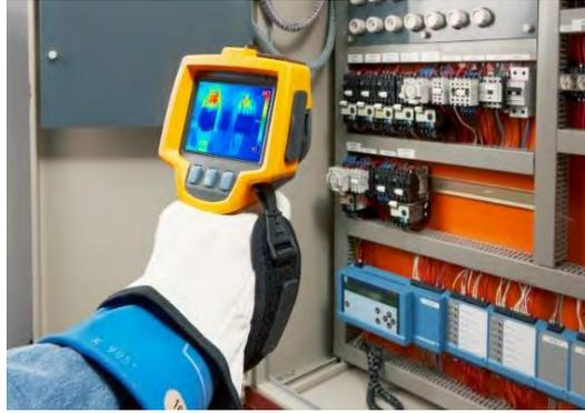
**Gambar 3. 28 Thermography Test**
