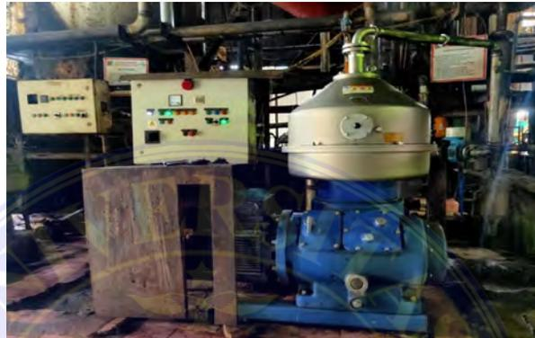
Gambar 3. 32. Sludge Seperator
